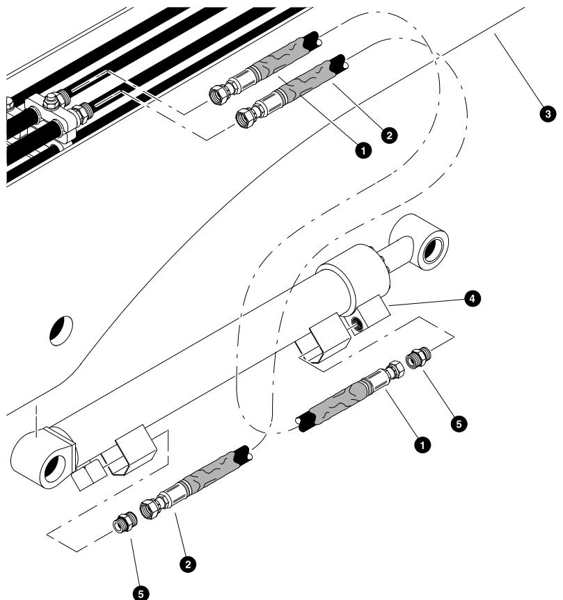
Main boom hoseline connections as viewed from the nose of the main boom looking towards the rear of the machine.
